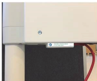
Figure 3-1. Power socket and power cable. Note the label showing Mains.
